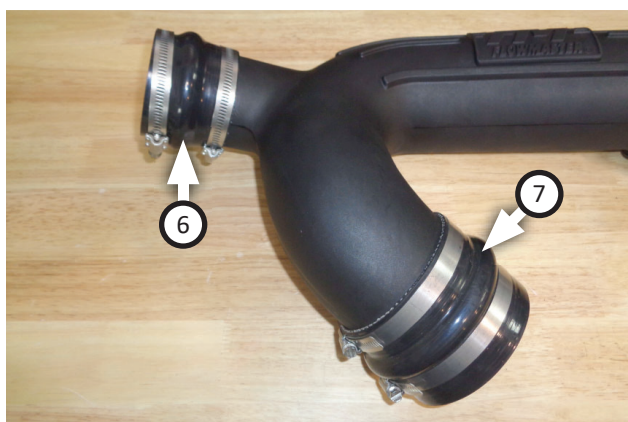
13. Slip (x2) clamps (8) onto hump coupler (6) . Slip (x2) clamps (9) onto hump coupler (7) . Push each coupler onto intake tube and partially tighten clamps.
