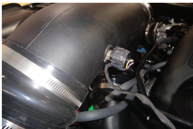
20. Carefully push inlet air temperature sensor into grommet and point locking tab toward air filter. Reinstall sensor plug and verify that connection is secure.
