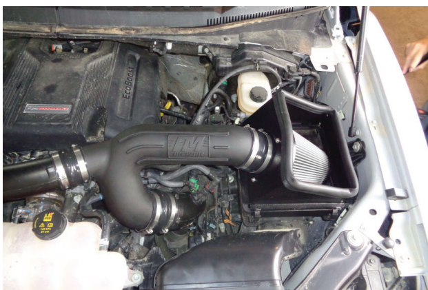
17. Insert (x4) airbox tabs on airbox into bracket, then lower assembly and connect (x2) couplers into turbo ducts. Do not tighten clamps.
