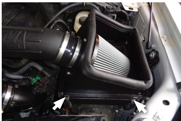
18. Secure airbox to bracket with (x2) latches.
