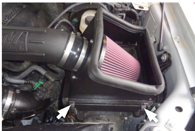
18. Secure airbox to bracket with (x2) latches.
