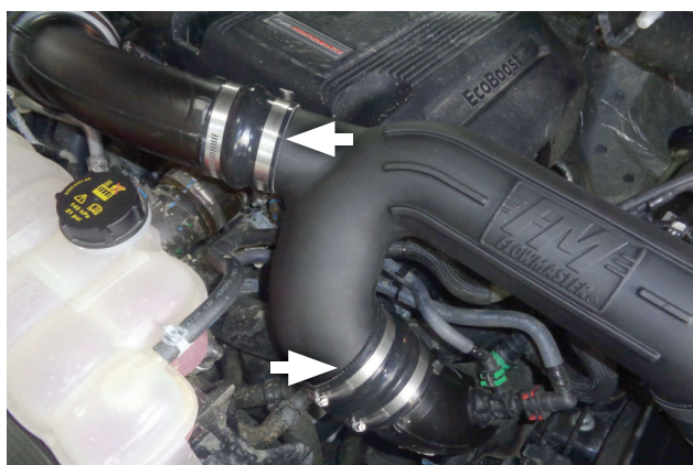
19. Push each coupler up against stops on turbo duct then tighten clamp. Center intake tube between all couplers, so there are approximately equal amounts of tube inserted in each coupler. Then tighten (x3) clamps on intake tube.
