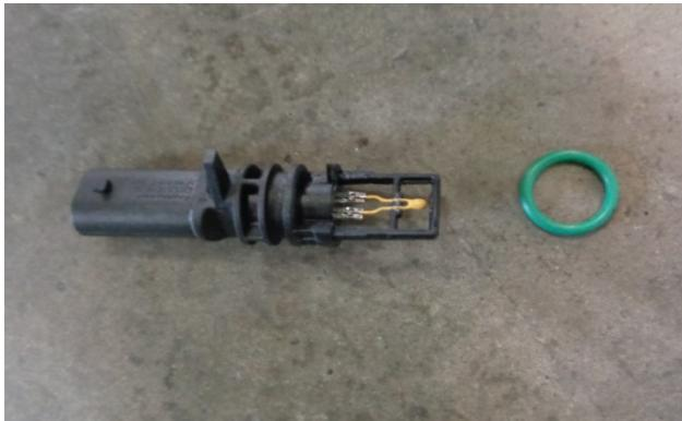
6. Remove the o-ring from the air temperature sensor. Place a sensor-safe grease or lubricant on the o-ring surface to facilitate easier installation into the FM air intake tube grommet. Retain in a safe location.
