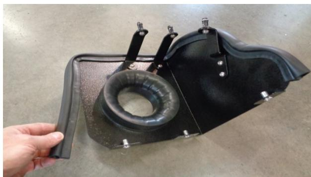
10. Install the rubber trim seal along the outer top and side edges as shown. Press fully into the groove starting from one end. Trim final length with metal shears for proper fitment.
