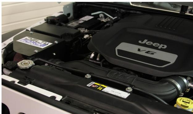
17. Secure the provided cone filter using the included hose clamp in the desired position. If desired, install pre-filter over the cone element. This will help extend the life of the filter by keeping out the larger particles. Using the last three  $\frac{1}{4}$ " screws/washers, secure the air-box lid, re-install the engine cover and the battery cable.
