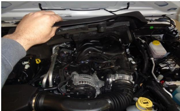
2. Remove the engine cover by grasping the front edge and lifting up, then pull forward. Unclip the coolant overflow hose from the air tube. *We highly recommend that customers retain their factory air intake system.*
