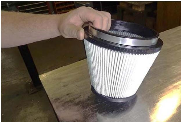
1. **Tap the filter** several times on a hard, flat surface. Tap it firmly enough to dislodge any loose particles from the pleats, but not so hard as to damage it.
