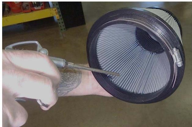
3. **Blow through** the filter, from the inside out. Keep the nozzle moving; do not hold it stationary over one place on the filter.
