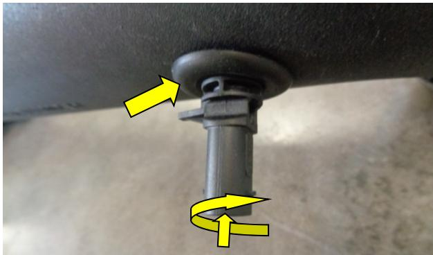
13. Insert the provided rubber grommet → into the hole in the FM intake tube. Insert the pre-lubed stock air temperature sensor into the grommet by twisting clockwise and pressing inwards until seated as above.
