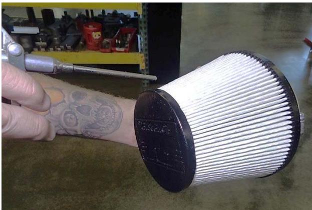
2. **Blow off the outside** of the filter. Blow across the filter surface (at about a 45° angle), not through the filter material. Hold the air nozzle about 6 inches away from the filter surface, always keep it moving, and point the air jet in to—not across—the pleats.
