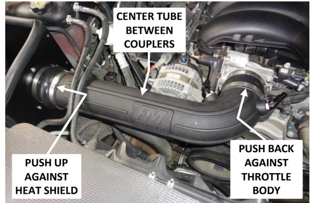
21. Install the intake tube in the vehicle. Push the rear coupler back against the throttle body and tighten the throttle body clamp. Push the left coupler up flush against the heat shield and tighten the heat shield clamp. Then center the tube between the couplers, and tighten both tube clamps.
