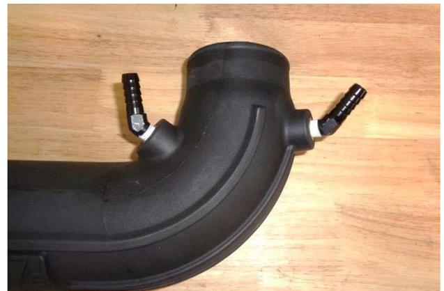
17. Apply 2 wraps of nylon thread tape to the threads of 2 barbed elbows (14), and install the elbows into the intake tube (13), pointing them toward the tube opening.
