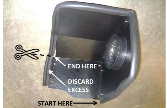
15. Attach the gasket (4) to the heat shield. Starting at the bottom of the front edge, firmly press the seal onto the edge, gradually working your way around. At the bottom of the opposite edge, trim the seal using metal-cutting shears.
