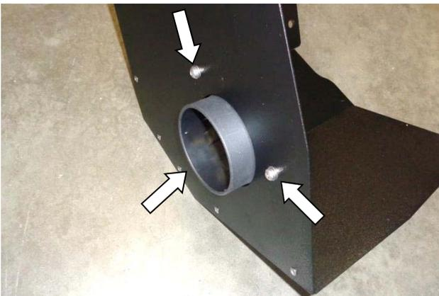
14. Assemble the air filter adapter (3) to the heat shield (5) using the M6 screws (8), lock washers (7) and flat washers (6).
