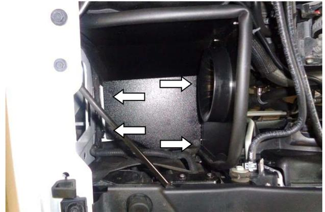
16. Use the 4 bolts retained at Step 12 to install the assembled heat shield in the vehicle. **NOTE: At each location, be sure to use the same length bolt as was removed (see Step 12).**
