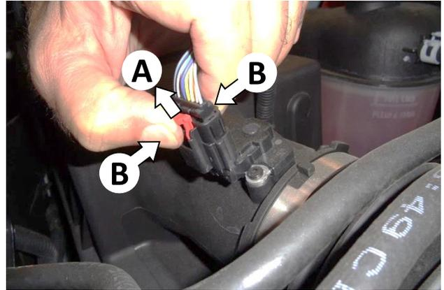
4. Disconnect the mass airflow (MAF) sensor plug by:
