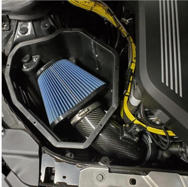
4) Attach the Intake Lid to the Airbox.
