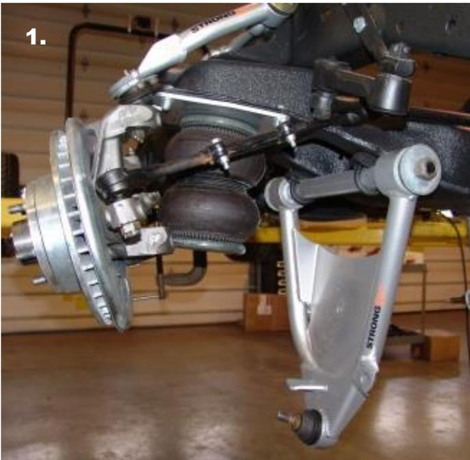
1. Bolt the lower Strong Arm to the frame using the OEM fasteners. The supplied cross shaft has 2 sets of holes. This CoolRide control arm uses the set of holes that are **8.705"** center to center. **Image 2** illustrates the holes used. Make sure to align the dowel in the frame with one of the holes in the cross shaft that is **8.705"** apart.
