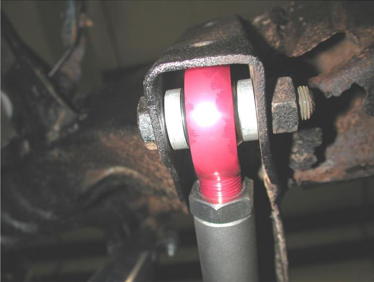
1. Install the  $\frac{3}{4}$ " jam nut onto the end of the Heim end, then screw Heim end into the end of the panhard bar.
