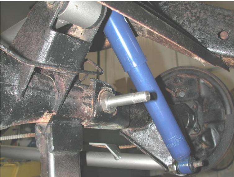
3. Bolt the new panhard bar stud onto the axle in factory stud location using the  $\frac{9}{16}$ " Nylok nut and flat washer supplied.
