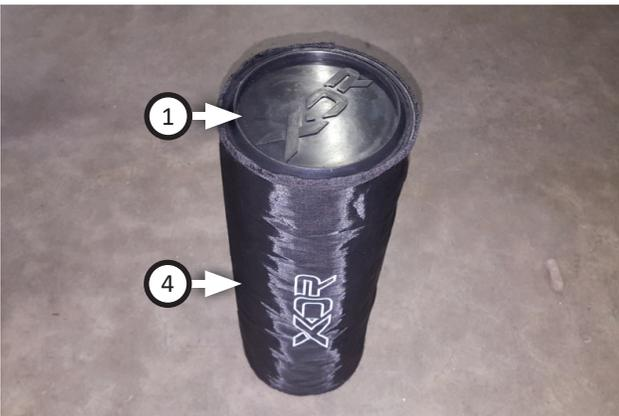
20. Fit **prefilter wrap (4)** over oiled air filter (1).
