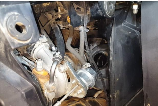
8. Remove intake tube top completely from vehicle.
