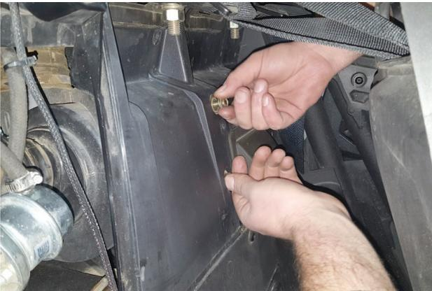
7. Behind drivers seat, remove (x2) fasteners securing factory airbox in place. Retain them for later.
