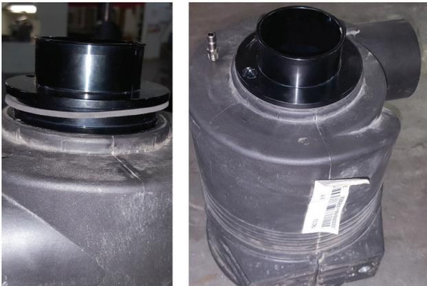
13. Wipe airbox clean, place coupler seal onto coupler then install to airbox, orienting threaded hole of coupler as shown.
