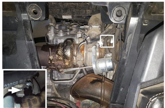
5. Loosen screw clamp and remove PCV hose from intake tube.
