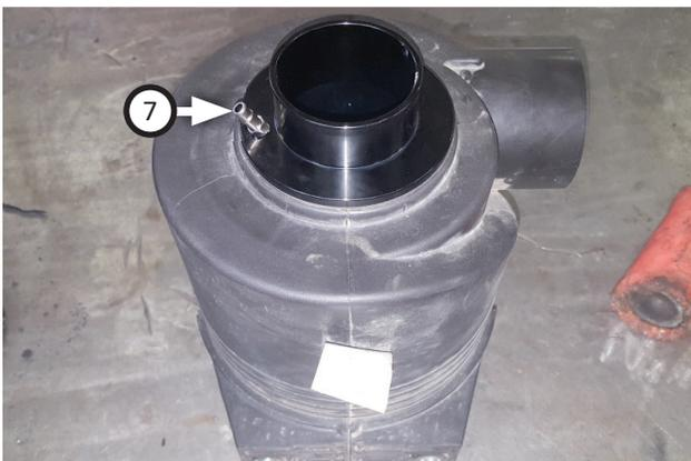
14. Install **straight connector (7)** into coupler as shown.
