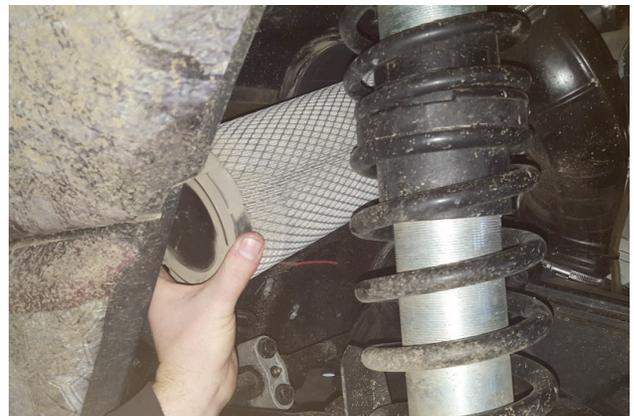
4. Remove factory air filter from vehicle.
