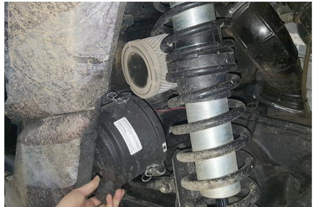
3. Unlatch then remove air filter cover (just forward of driver rear tire).
