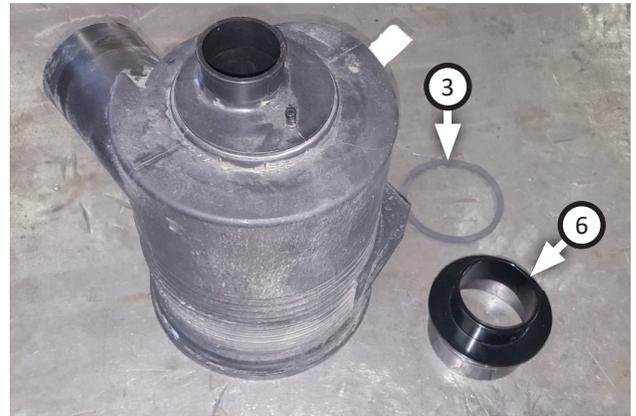
10. Bring airbox to work bench, along with coupler (3) and coupler seal (6).
