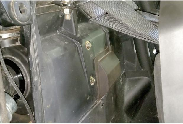
18. Secure factory airbox in place by re-installing (x2) bolts (removed step 7) behind driver seat.
