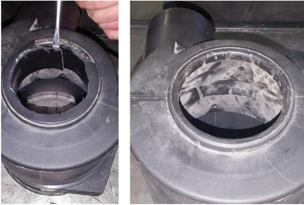
12. Now remove remaining rim from airbox without breaking tabs beneath.
