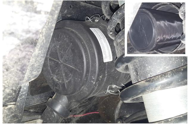
21. Set filter into factory intake tube then replace air filter cover (removed step 3) and latch it in place.
