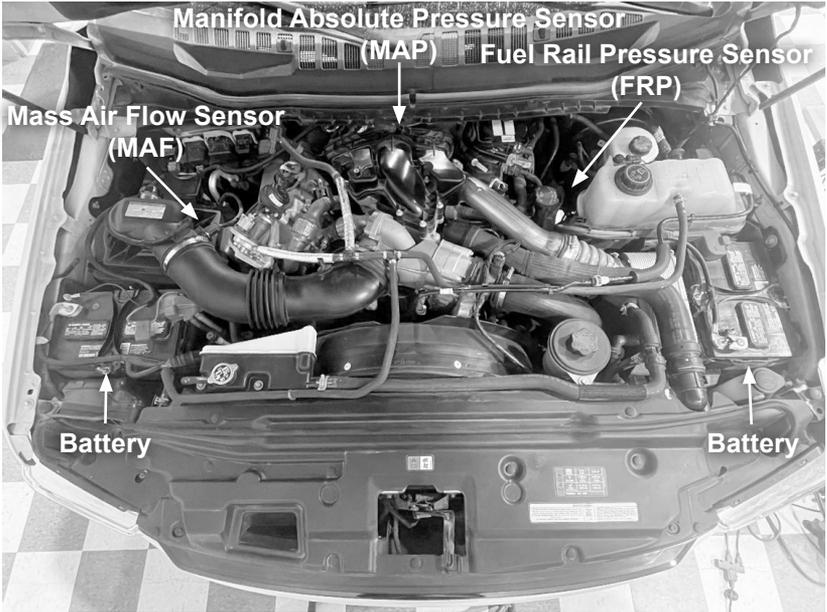
**STEP 2** - Locate the MAF connector on the intake box, and disconnect it by sliding the locking tab up, then squeezing the release tab. Connect both connectors to the EZX harness.
