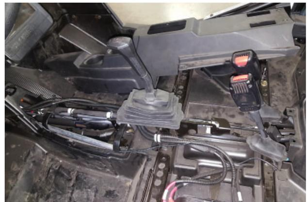
5. Fit rubber boot into center then lift and remove console cover.
