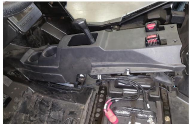
4. Shift into NEUTRAL, then remove console fasteners (x7) and retain them for later use.
