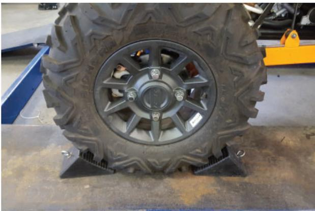
2. Securely chock vehicle's wheels to keep it from rolling while shift lever is being manipulated.
