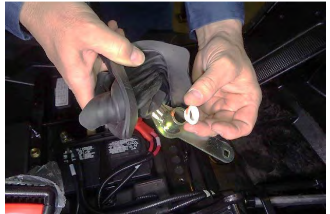
12. Remove and retain the two bushings.
