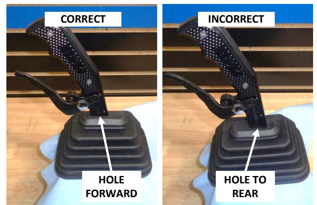
13. Ensure that the boot is oriented on the shift lever with the hole facing forward. If not, orient the boot correctly by carefully rotating it around the lever.
