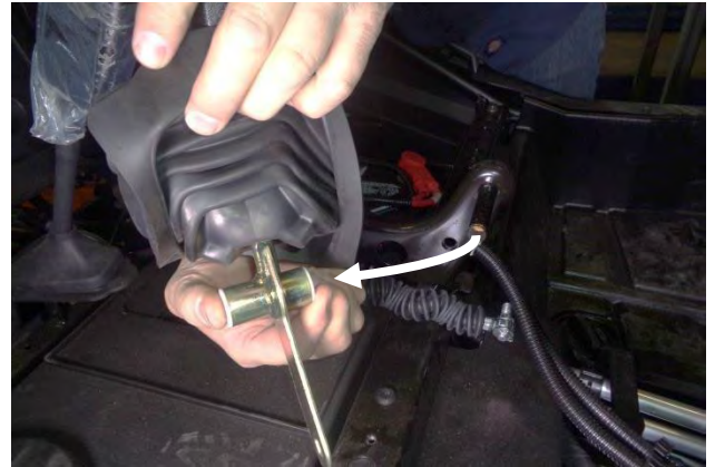
11. Remove the shift lever from the pivot shaft, taking care not to lose the nylon bushings in each end of the bore.
