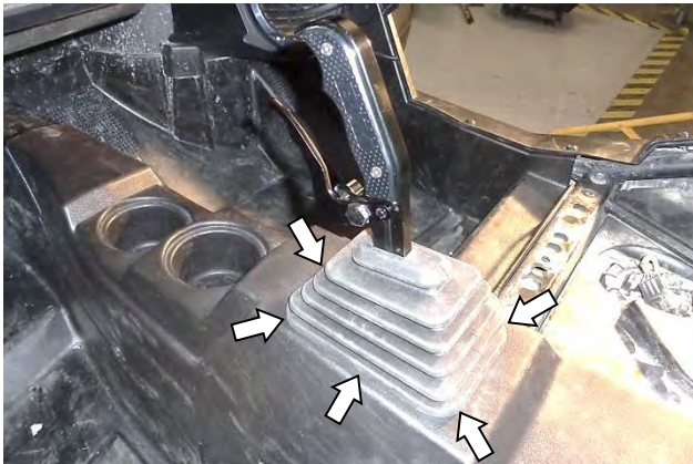
26. Carefully pull the shifter boot upward until its groove fully engages the console opening.
