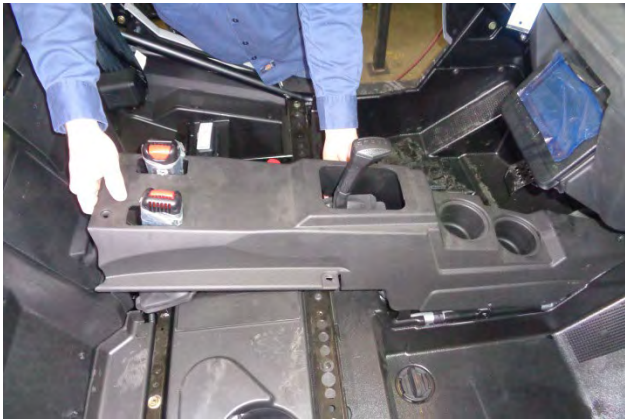
8. Remove the center console from the vehicle.
