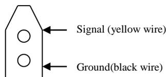
Connect the yellow wire to the tach output signal from the ignition box. Connect the black wire to ground.
