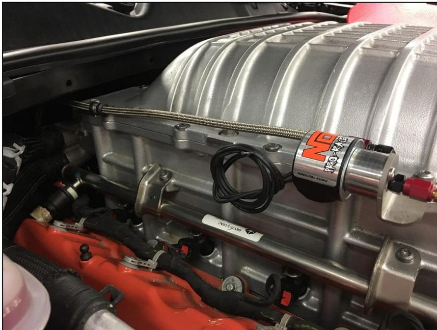
**Figure 18 – Assembled Fuel Supply Hose and Fuel Solenoid**
