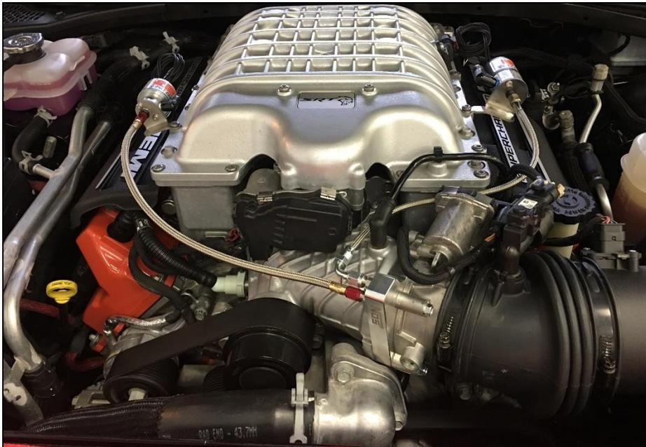
**Figure 11 – Nitrous and Fuel Hose Routing**
