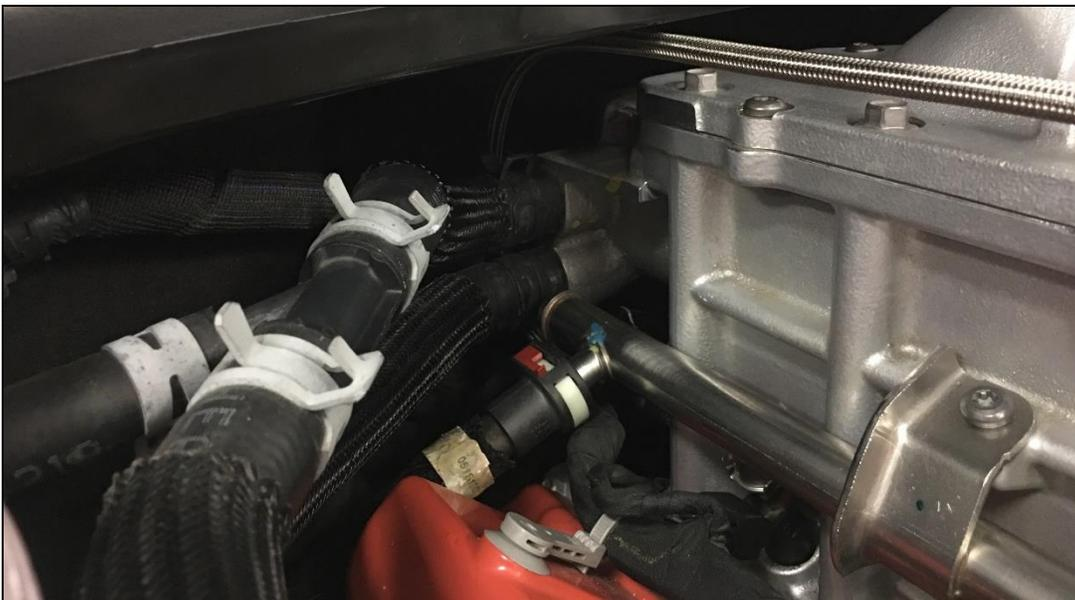
**Figure 17 – Reassembled Fuel Rail and Hose Routing**
