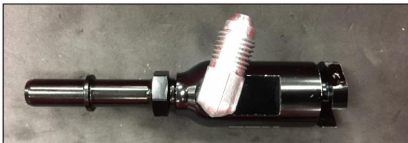
**Figure 12 – Fuel Tap Adapter Orientation**
