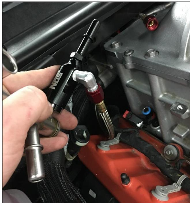
**Figure 15 – Fuel Tap to OE Fuel Rail Assembly**
