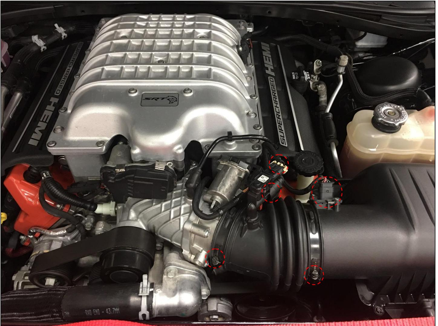
**Figure 6 – Intake Air Tube Removal**
